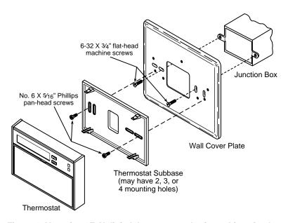
Figure 1. Mounting 1F9X digital thermostat to horizontal junction box
